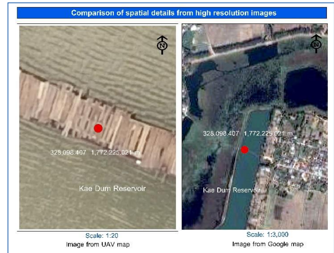
Figure 6. Detail comparison from high-resolution images of the same position on the bridge section C
